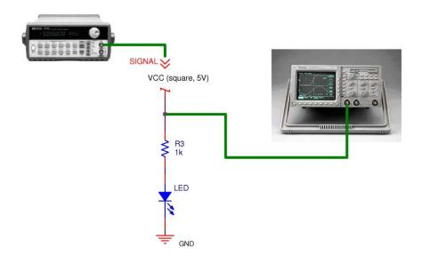
The signal generator must provide 5V p-p (peak-to-peak) from TTL/SYNC output.
