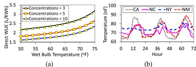
Fig. 1. (a) Direct WUE versus outside wet bulb temperature [44]. Lines/markers represent modeled/measured values. (b) 3-day outside temperature starting from July 1, 2012 [11].
