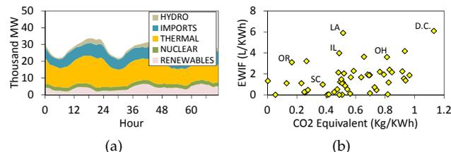
Fig. 2. (a) 3-day fuel mix data of California ISO starting from Sep 1, 2013 [1]. (b) State-level EWIF versus CO<sub>2</sub> emissions in the U.S. [45], [47].
