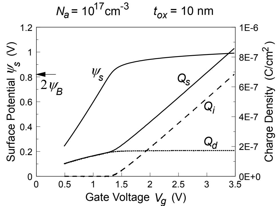
Gate voltage equation ( $V_{fb}=0$ ):
