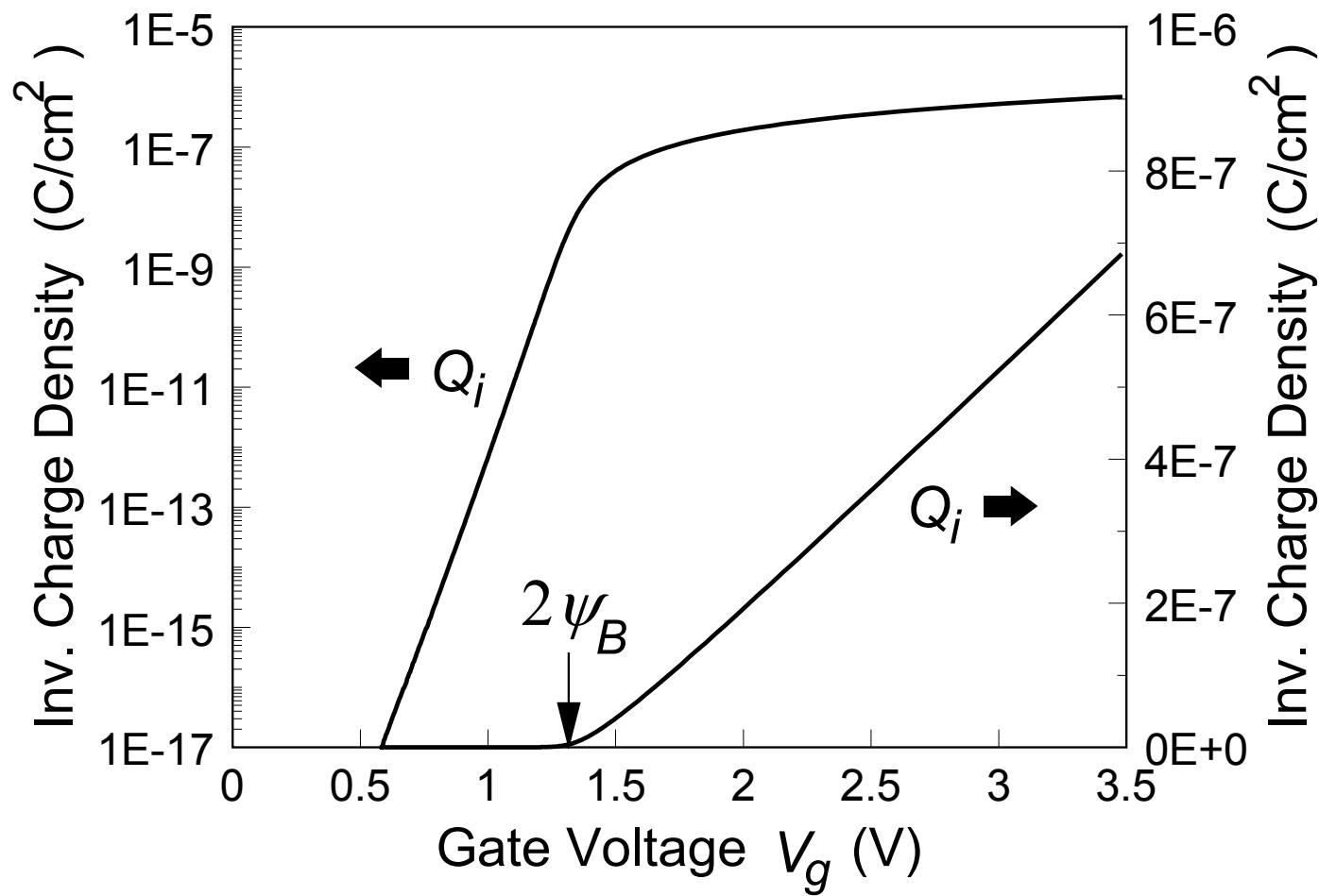
$$N_a = 10^{17} \text{ cm}^{-3} \quad t_{ox} = 10 \text{ nm}$$
