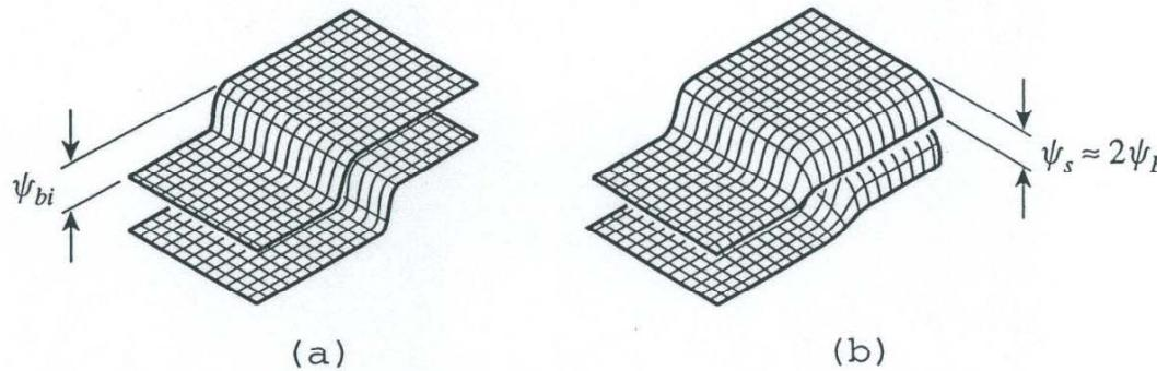
The electron quasi-Fermi level in the MOS is the same as the Fermi level of the p-type Si.
