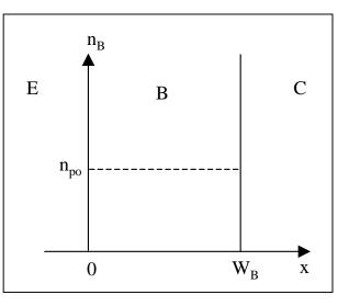
8. For an npn BJT at T=300K with a base width of 0.05  $\mu$ m and a minority electron mobility in the base of 800 cm<sup>2</sup>/Vs, what is the maximum value for the transition frequency, f<sub>T</sub>?
