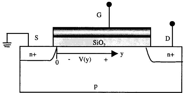
$$\int_0^{V(y)} W \mu_n Cox Q_n(v) = \int_0^y dy = I_D$$
