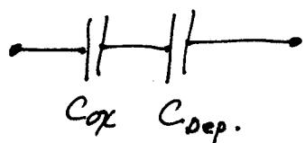
$$C_{ox} = \frac{\epsilon_{ox}}{t_{ox}} \quad C_{oep} = \frac{\epsilon_s}{W_0}$$
