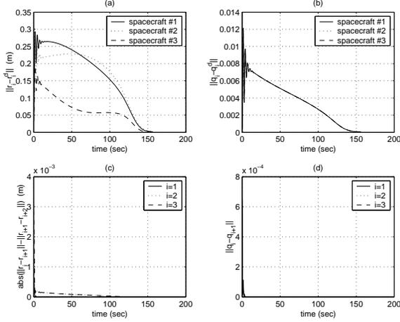
Figure 3: Position and attitude errors with formation feedback (convergence time: 156 sec).
