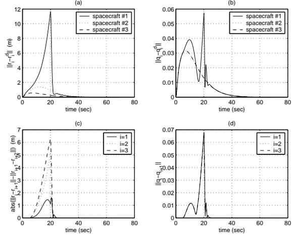
Figure 4: Position and attitude errors without formation feedback when spacecraft #1 fails for 15 seconds (convergence time: 69 sec).
