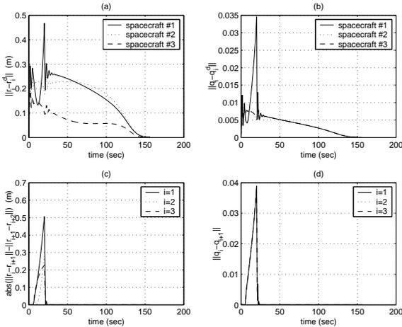
Figure 5: Position and attitude errors with formation feedback when spacecraft #1 fails for 15 seconds (convergence time: 156 sec).
