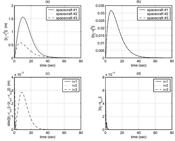
Figure 2: Position and attitude errors without formation feedback (convergence time: 69 sec).
