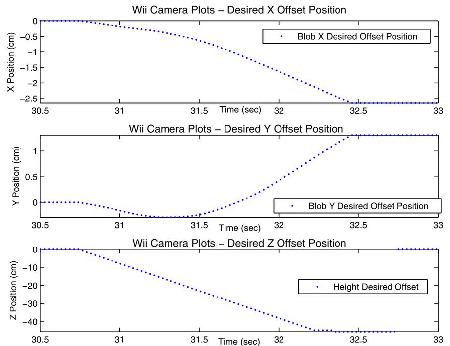
**Fig. 24** Desired and actual positions of the quadrotor as seen by the navigation controller, in  $x$  and  $y$ . The blob is seen by the IR camera at 30.7 sec, at which point the desired positions (in red) are adjusted by the desired offsets, and gripping is activated at about 32.4 sec. After gripping, the navigation controller returns to a hover mode (Color figure online)
