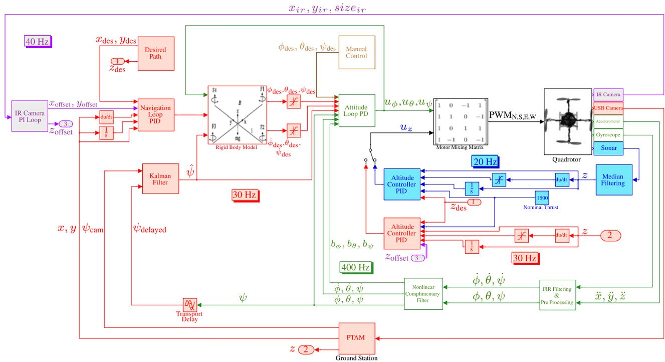
**Fig. 7** Control block diagram. The green blocks indicate the attitude control system; the blue blocks are for the sonar altitude controller; red indicates the navigation system utilizing the SLAM algorithm on the
