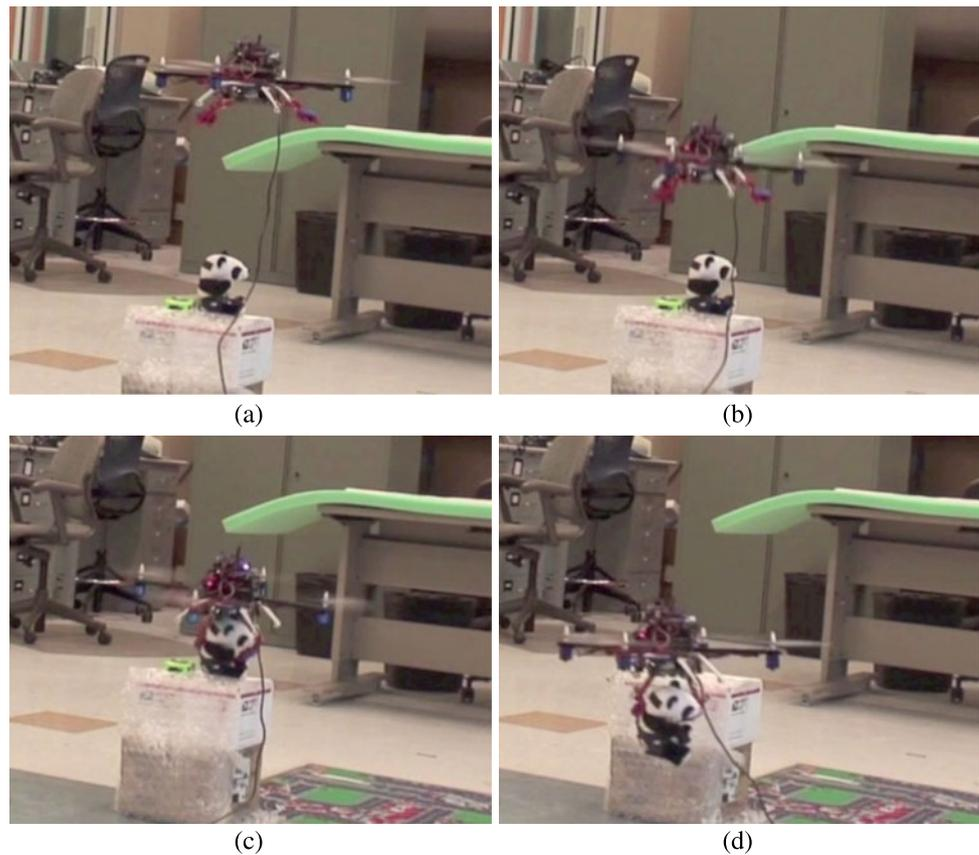
ing the possible issues described above. Gripping is kept simple by means of just an extra sensor and an upper feedback controller over the navigation system in order to reduce the error seen by the camera without requiring camera calibration for absolute measurement information.
