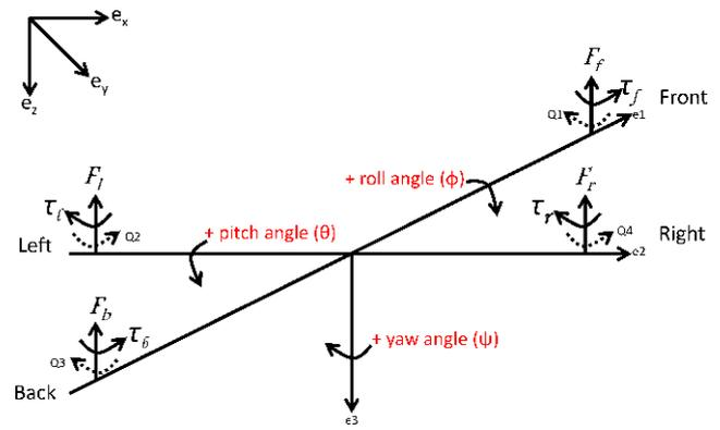
**Fig. 2** Model of a quadrotor
