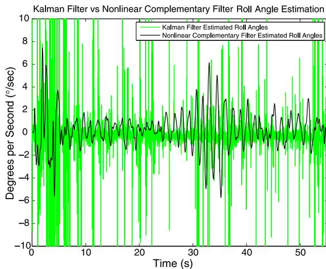
**Fig. 6** Comparison of the attitude of the quadrotor, for the roll angle, extracted using the nonlinear passive complementary filter and the Kalman filter. This data is from a typical hover flight maintained using vision-based navigation
