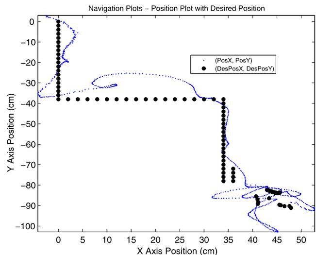
**Fig. 22** Coordinate plot showing the quadrotor navigating to the object. Takeoff occurs in the *upper left quadrant* of the graph, with gripping occurring in the *lower right*. Way-points were given incrementally to the quadrotor until gripping was activated over the object
