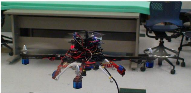
**Fig. 1** The quadrotor, in flight, used to perform aerial gripping
