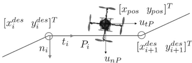
**Fig. 8** Path definition, with way-points  $i$  and  $i + 1$  and corresponding path segments, noting the tangent and normal path components
