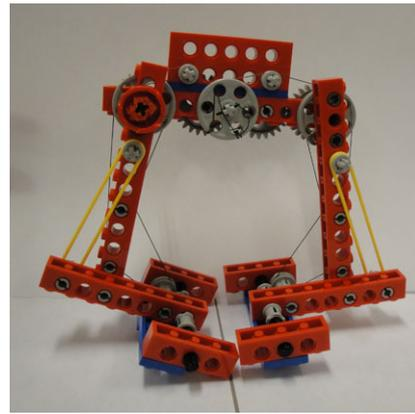
**Fig. 12** Gripper showing the cables, pulleys and elastic bands used to provide compliance and under-actuation
