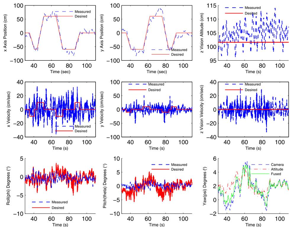
The quadrotor was able to keep a hover within  $\pm 20$  cm after lowering the gains as can be seen in Fig. 18. This specific flight is with the fan blowing only in the direction of the  $x$
