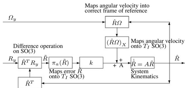
Fig. 5 Block diagram of the nonlinear complementary filter
