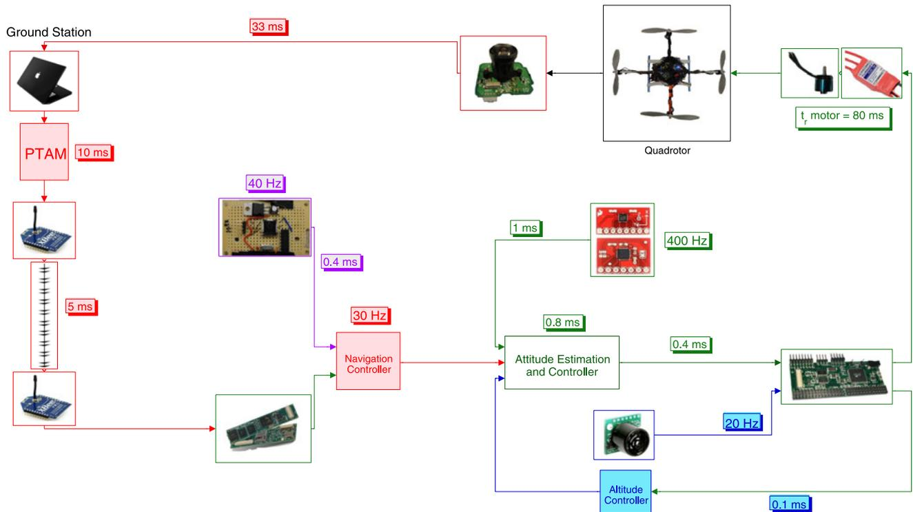
**Fig. 4** Quadrotor system latency diagram by component and communication. The green blocks indicate the attitude control system; the blue blocks are for the sonar altitude controller; red indicates the navigation
