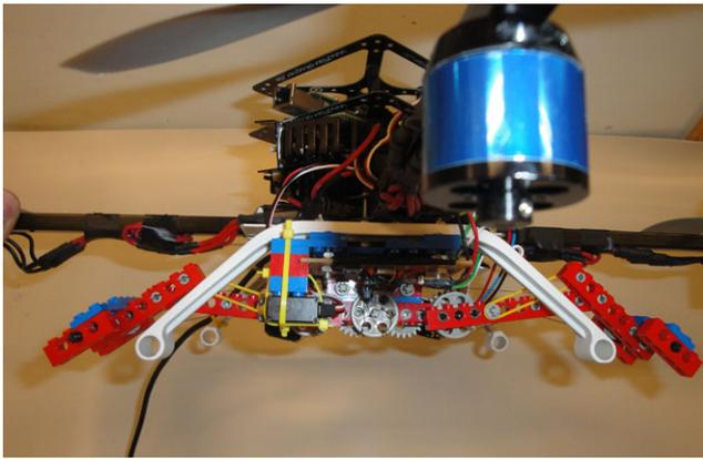
**Fig. 13** Gripper shown mounted under the quadrotor
