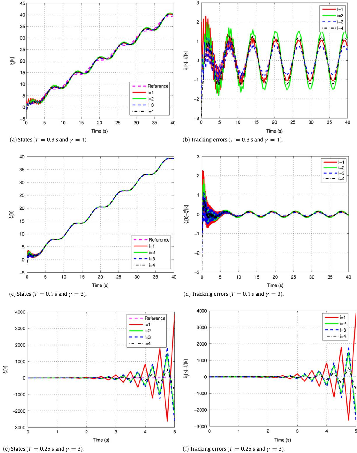
Fig. 2. Distributed discrete-time coordinated tracking using PD-like discrete-time consensus algorithm (5) under different  $T$  and  $\gamma$ .
