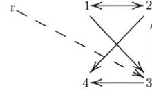
**Fig. 1.** Directed graph for four vehicles. A solid arrow from  $j$  to  $i$  denotes that vehicle  $i$  can receive information from vehicle  $j$ . A dashed arrow from  $r$  to  $l$  denotes that vehicle  $l$  can receive information from the virtual leader.
