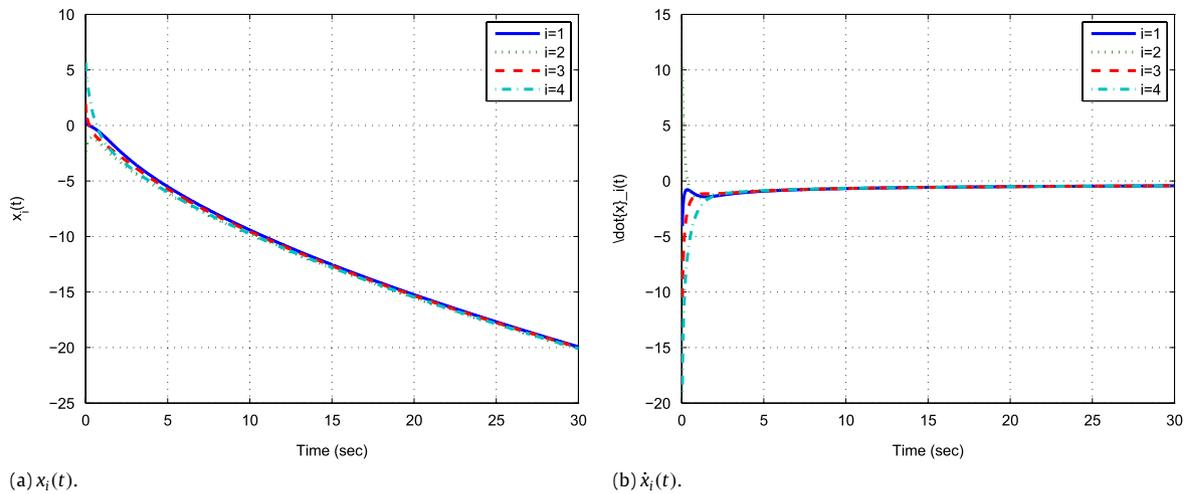
Fig. 5. States of the four systems using (22) with  $\alpha = 1.2$  and  $\gamma = 1$  with the directed fixed network topology given by Fig. 3.
