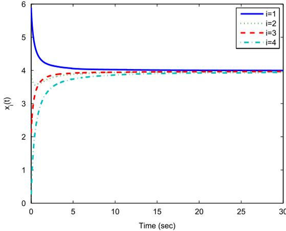
**Fig. 2.** States of the four systems using (5) when the network topology switches between Fig. 1(a) and (b) every 3 s with  $\alpha = 0.8$ .
