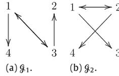
**Fig. 1.** Directed network topology for four systems. An arrow from  $j$  to  $i$  denotes that system  $i$  can receive information from system  $j$ .
