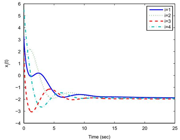
**Fig. 4.** States of the four systems using (16) with  $\alpha = 1.6$  and  $\beta = 1$  with the directed fixed network topology given by Fig. 3.
