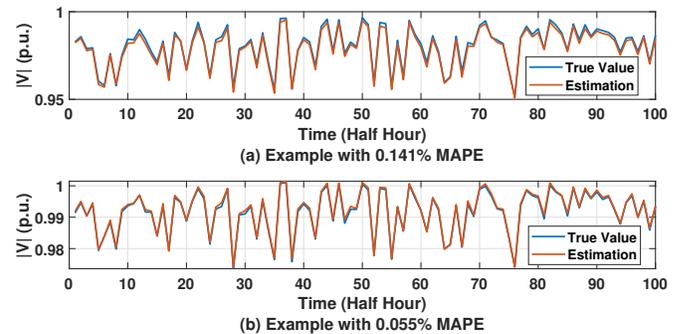
Fig. 3. Examples of voltage estimation.
