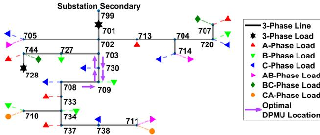
Fig. 1. Schematic of a modified IEEE 37-bus test feeder.
