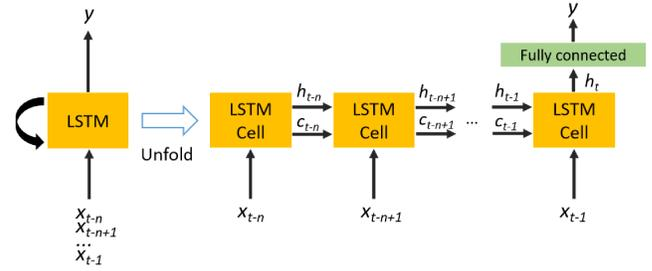
Fig. 1: Unfolded computational graph of an LSTM.
