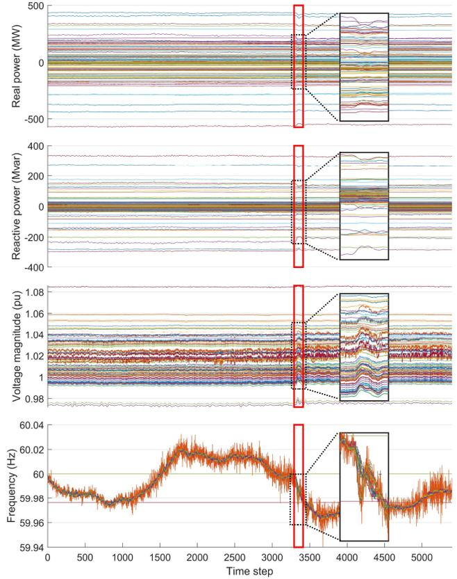
Fig. 3: PQ|V|f data of a sample frequency event.
