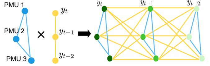
Fig. 2: Product graph construction for PMU data streams.
