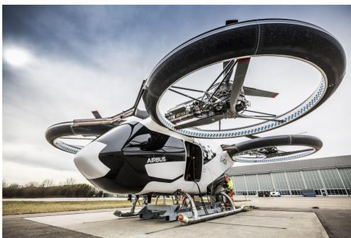
**Fig. 3 The CityAirbus eVTOL aircraft**
