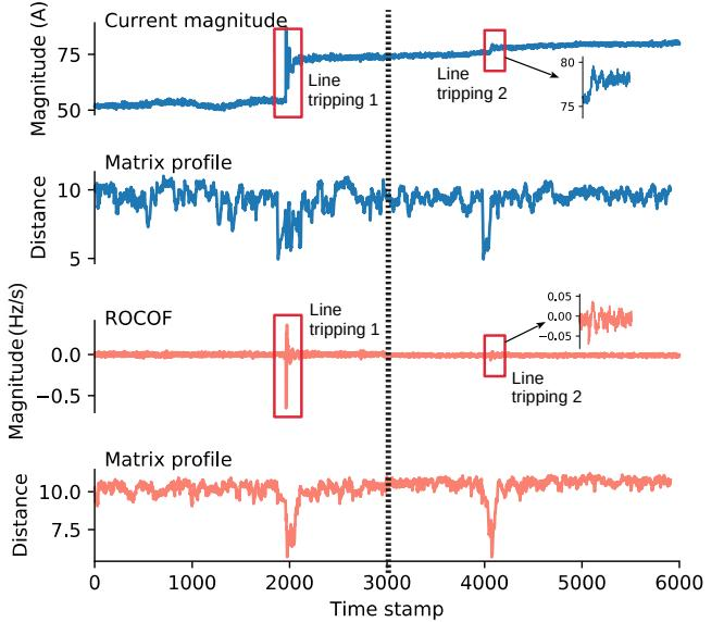
Fig. 3: Current magnitude and ROCOF time series from line tripping event file and their matrix profiles.
