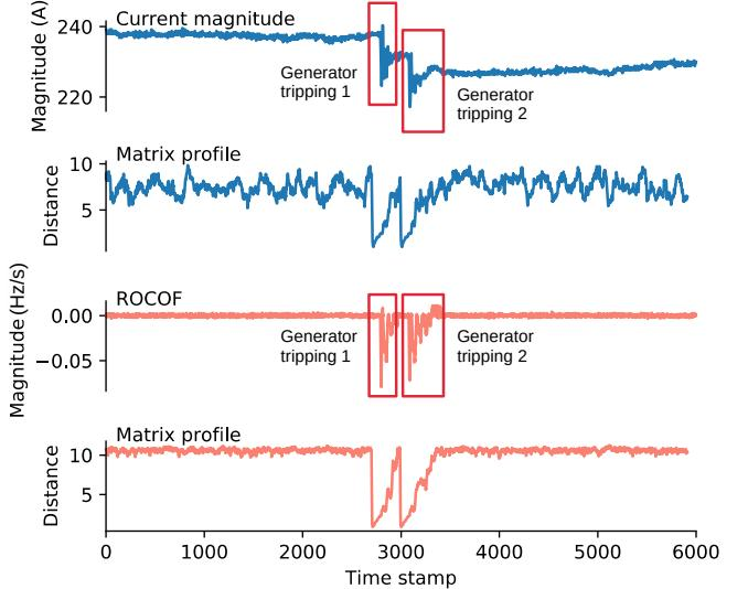
Fig. 2: Current magnitude and ROCOF time series from generator tripping event file and their matrix profiles.
