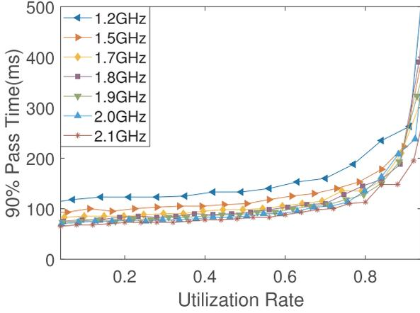
Fig. 5. 90% pass time versus utilization rate.
