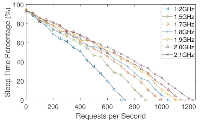
Fig. 3. C6 sleep time versus request per second rate.
