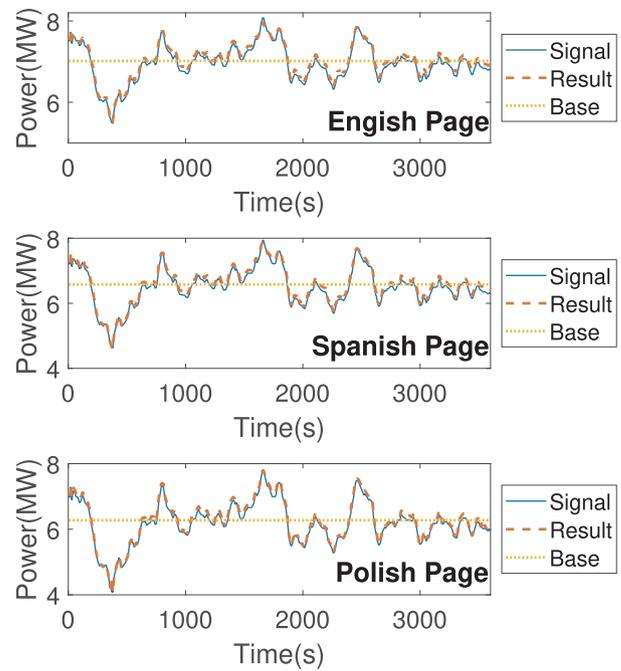
**Fig. 9.** Frequency regulation signal following of one hour for the three different pages.
