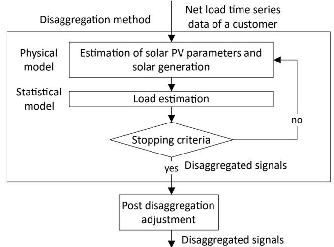
Fig. 1. The overall framework for disaggregating net load of residential customers with solar PV systems.
