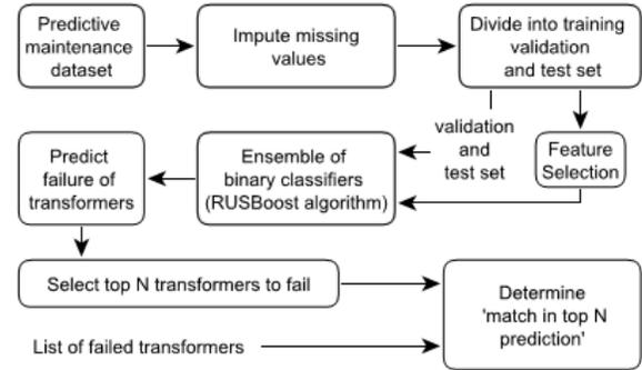
Fig. 1: Workflow for failure prediction of distribution transformers
