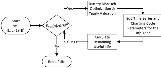
Fig. 1: Battery lifetime valuation framework
