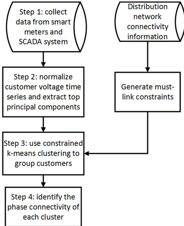
Fig. 2: Diagram of the phase identification procedure.
