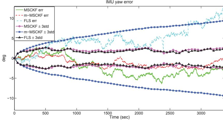
Figure 1: IMU yaw errors and  $\pm 3\sigma$  bounds in one representative trial. The yaw error for the MSCKF (solid line – green), the m-MSCKF (dashed line – red), and the FLS (dashdot line – cyan). The  $\pm 3\sigma$  bounds for the MSCKF (circles – magenta), the m-MSCKF (squares – blue), and the FLS (triangles – black).
