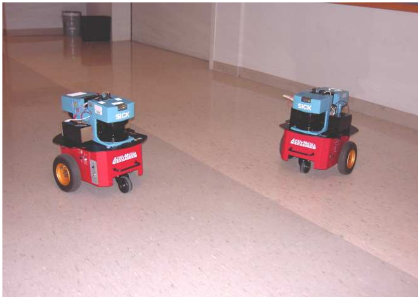
Figure 2.9: The Pioneer III robots used in the experiments. Two laser range-finders are installed on each robot, to provide a 360° field of view.
