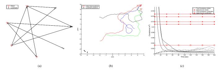
Fig. 1. (a) The RPMG used for the simulation experiments (b) The initial positions and part of the trajectories of the robots for an adverse C-SLAM scenario. (c) Comparison of the actual covariance of the position estimates against the worst-case performance bound, for the scenario in (b). The plotted lines correspond to the mean of the covariance along the two coordinate axes.
