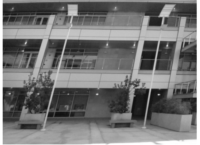
Fig. 1: An example image with rolling-shutter distortion.
