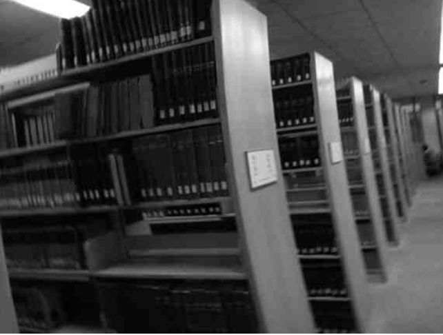
Fig. 10: A sample image from the indoor experiment, showing significant rolling-shutter distortion.
