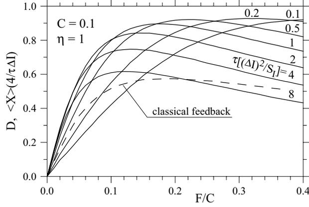
**Figure 4.** Dependence of the synchronization degree  $D$  on the feedback factor  $F$  in ideal case ( $\gamma = 0$ ) for several  $\tau$ . Experimentally  $D$  can be measured via average in-phase current quadrature  $\langle X \rangle$ . Dashed line is for a classical feedback.
