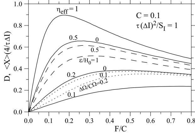
**Figure 5.** Solid lines: synchronization degree  $D$  (and in-phase current quadrature  $\langle X \rangle$ ) as functions of  $F$  for several values of the detection efficiency  $\eta_{\text{eff}}$ . Dashed and dotted lines illustrate the effects of the energy mismatch ( $\varepsilon \neq 0$ ) and the frequency mismatch ( $\Omega \neq \Omega_0$ ).
