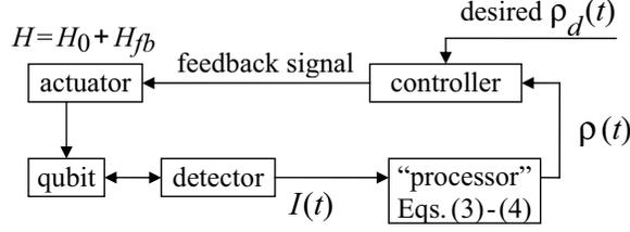
**Figure 1.** Schematic of the Bayesian quantum feedback loop which maintains quantum coherent oscillations in a qubit for arbitrarily long time. Real-time solution of quantum Bayesian equations by the “processor” provides exact monitoring of the qubit density matrix  $\rho$ . Qubit tunneling amplitude  $H$  is controlled depending on the difference between  $\rho(t)$  and the desired qubit evolution  $\rho_d(t)$ .
