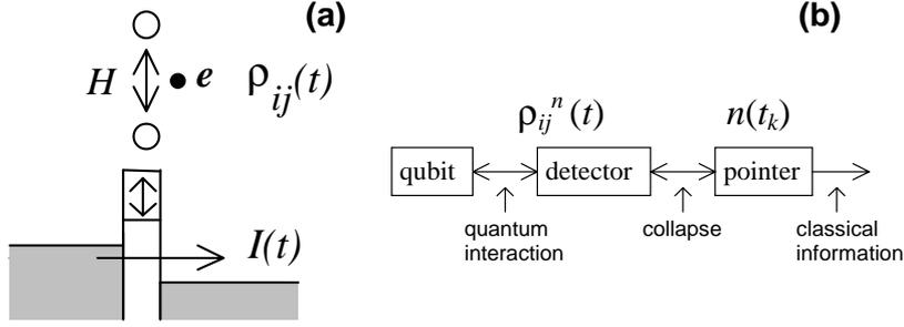
**Figure 2.** (a) Tunnel junction as a detector of the double-quantum-dot qubit. The electron location in the DQD affects the detector barrier height. The noisy current  $I(t)$  (detector output) reflects the evolution of the qubit density matrix  $\rho_{ij}(t)$ . (b) Idea of the Bayesian formalism derivation via Bloch equations. The number  $n$  of electrons passed through the detector is periodically collapsed (forced to choose a definite value) at moments  $t_k$ .
