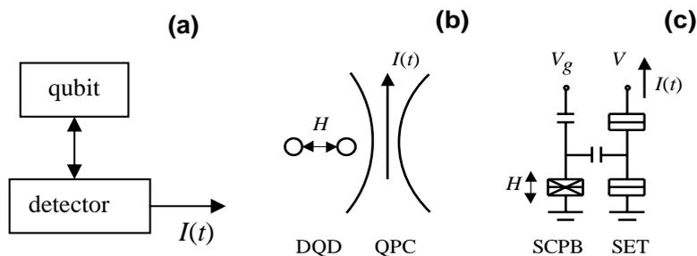
**Figure 1.** (a) General schematic of a continuously measured solid-state qubit and two particular realizations of the setup: (b) a qubit made of double quantum dot (DQD) measured by a quantum point contact (QPC) and (c) a qubit based on single-Cooper-pair box (SCPB) measured by a single-electron transistor (SET).
