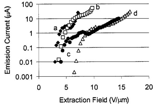
FIG. 7.  $I$ - $E_0$  results for (a) carbon black/silica/photoresist, (b) carbon nanotubes/photoresist, (c) untreated diesel exhaust/photoresist, and (d) carbon black/photoresist samples measured at 120 °C.
