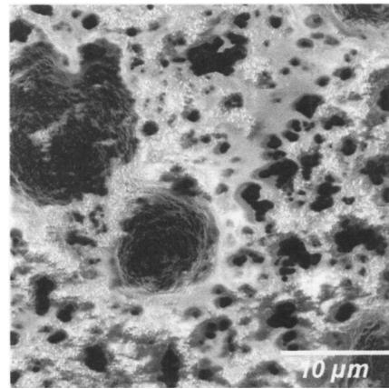
FIG. 3. SEM image of the top view of carbon black and silica dispersed in Shipley S1818 photoresist after baking in air at 120 °C. Carbon/silica islands form between photoresist islands. The packing density depends on the volume fraction of the carbon black/silica powders.
