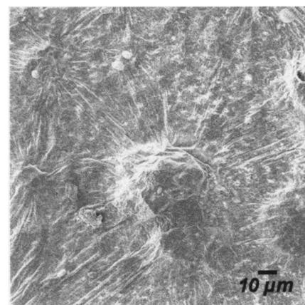
FIG. 4. SEM image of untreated diesel exhaust dispersed in Shipley S1818 photoresist after baking in air at 120 °C.
