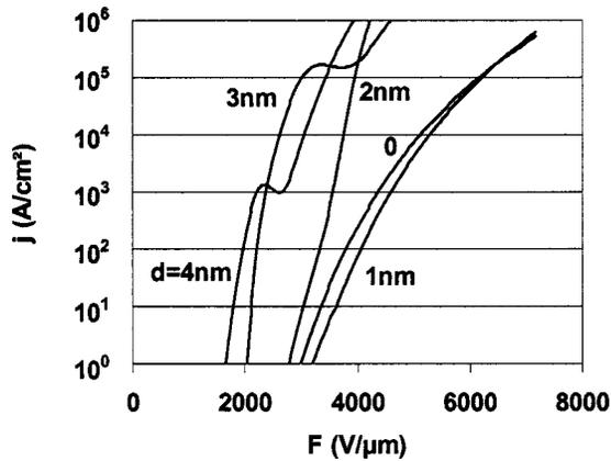
FIG. 8. Theoretical  $j$ - $F$  curves for barrier layer thicknesses of 0, 1, 2, 3, and 4 nm using the rF-N tunneling model (presented in Ref. 11).
