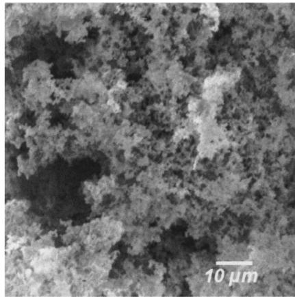
FIG. 1. SEM image of the top view of carbon black and silica dispersed in isopropanol after the isopropanol evaporated.
