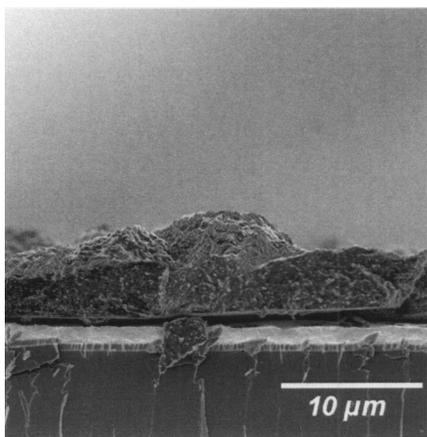
FIG. 2. SEM image of the cross section of carbon black and silica dispersed in Shipley S1818 photoresist. The film is deposited onto a copper-coated silicon substrate and baked in air at 120 °C.
