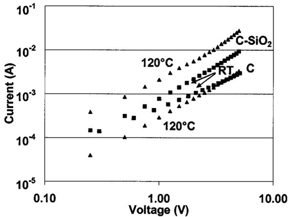
FIG. 5.  $I$ - $V$  curves of carbon black/photoresist and carbon black/silica/photoresist samples in the vertical direction. The measurements were performed at RT and at 120 °C.
