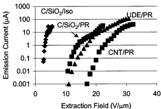
FIG. 6.  $I$ - $E_0$  results for carbon black/silica/isopropanol, carbon black/silica/photoresist, untreated diesel exhaust/photoresist, and carbon nanotubes/photoresist samples measured at room temperature.
