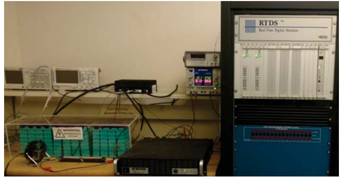
Fig. 1. The power hardware in loop (P-HIL) testbed for the grid-connected battery storage system using RTDS Simulator and lab-scale battery cells.
