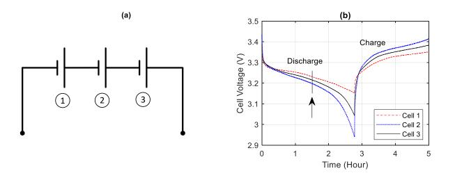
• The battery cells are initially charged, and they are balanced. Then they are discharged and subsequently charged. The cell voltages during the discharge and charge cycle are shown in Figure (b).
