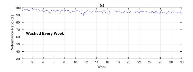
• Example 7.4 (Cont.): We see that the profiles for the performance ratio vary drastically across these three PV arrays. In particular, the power production may drop to as low as only 40% of the normal production rate under low wash conditions; while the power production is almost always close to the normal production rate under high wash conditions.
