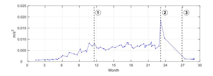
• After about six months, the vibration level started to gradually increase, suggesting potential issues with the main bearing.
