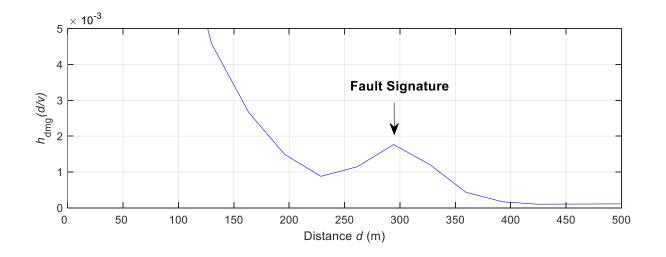
• Here, the damage impulse response is plotted over the *distance* that the communication wave travels, denoted by *d*. Let *v* denote the *propagation speed* of communication wave. We can express *time t* as follows:
