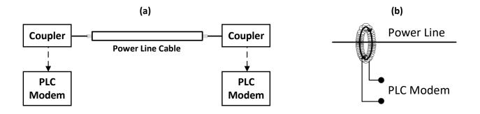
• At the transmitter, data is first modulated into a communication carrier signal by the modem. The *communication carrier signal* is then injected into the power line by a coupling device that acts as a PLC modem. At the receiver, the communication carrier signal is extracted from the power line by another coupling device that too acts as a PLC modem. The signal is then demodulated by the modem to obtain the original data.
