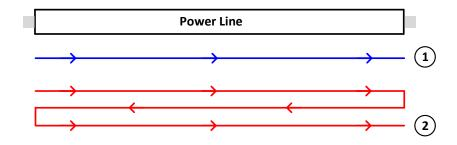
• Additional reflected signals arrive at the receiver, after four echos, six echos, and so on, although they are not shown in this figure. Reflected signals are attenuated more than the original signal because they travel longer through the power cable. Nevertheless, their impact must be addressed by using proper signal processing methods; cf. [412].
