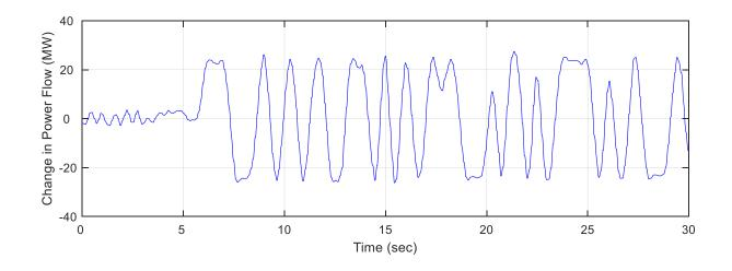
• This type of noise modulation probing signals can excite the power system across a range of local oscillation modes. The above probing signal in can *excite the system at frequencies from 0.1 Hz to 1.1 Hz*; see [403].
