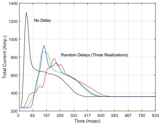
Fig. 5. Examples of the aggregate load transient profile under different delay scenarios. The regulation down event is assumed to occur at time zero.
