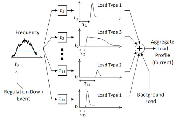
Fig. 4. The method of calculating the aggregate load current profile at a regulation down event under different load types and different delay values.
