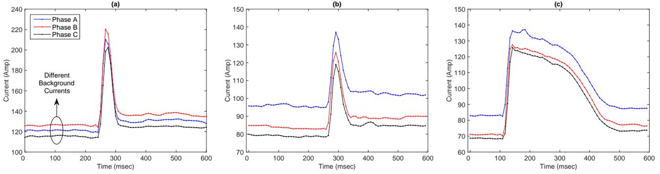
Fig. 3. The three *current surge signatures* that represent the three load types with significant current surges that are identified through analysis of  $\mu$ PMU data.
