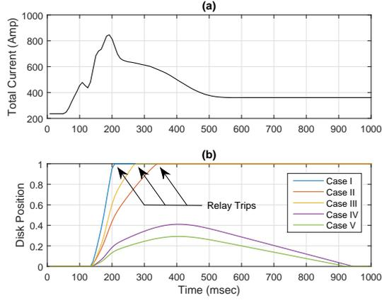
Fig. 7. Changes in relay disk position in response to a regulation down event induced aggregate surge current: (a) total surge current; (b) disk positions.
