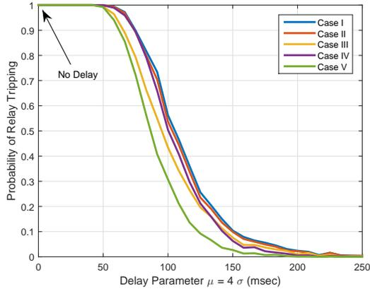
Fig. 8. Impact of delay distribution parameters on tripping probability.
