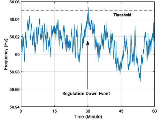
Fig. 1. A regulation down event occurs when frequency exceeds a threshold.
