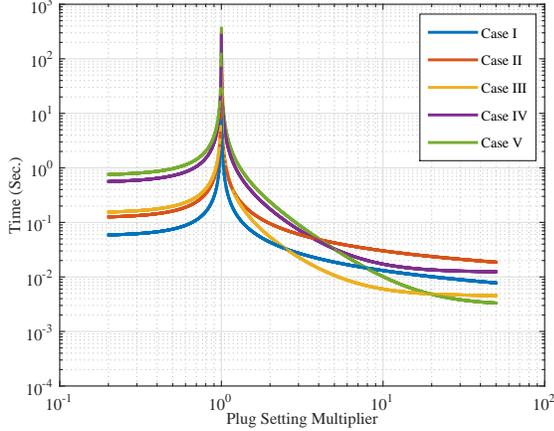
Fig. 6. The ITCCs of the different protection relays in Table I.
