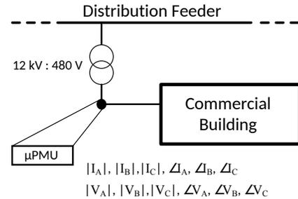
Fig. 2. Test system with a  $\mu$ PMU and its corresponding measurements.
