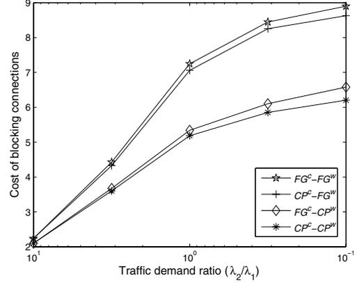
Fig. 2. Cost of blocking connections versus traffic demand ratio  $\lambda_2/\lambda_1$ .
