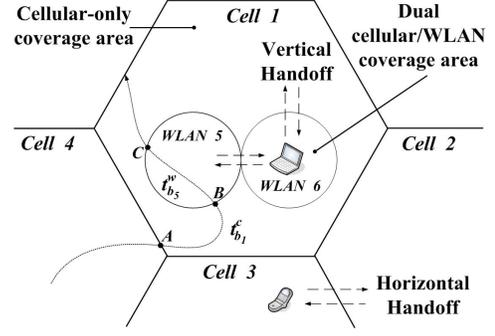
Fig. 1. An integrated multi-service cellular/WLAN system.
