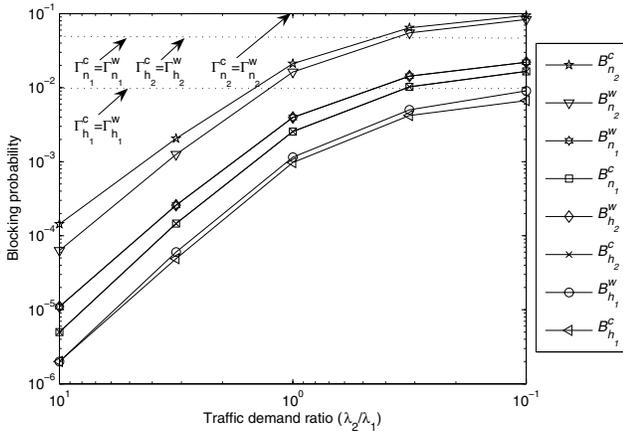
Fig. 4. New connection and handoff blocking probabilities for  $CP^c-CP^w$ .
