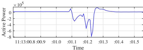
Fig. 6. Active power of phase C measured by Micro-PMU 1.
