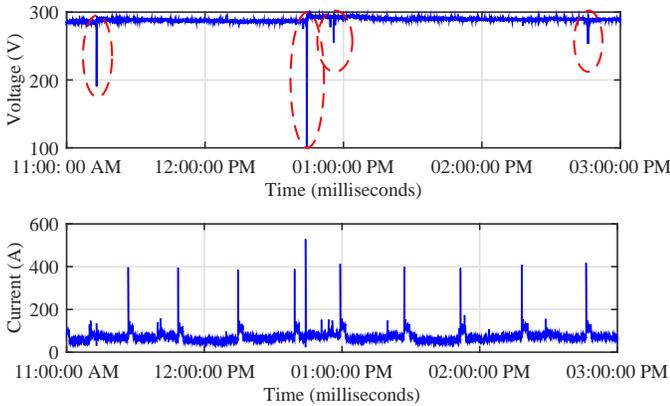
Fig. 2. Single phase voltage and current of Micro-PMU 3 for a four-hour period during a rainy day, October 24 2016.
