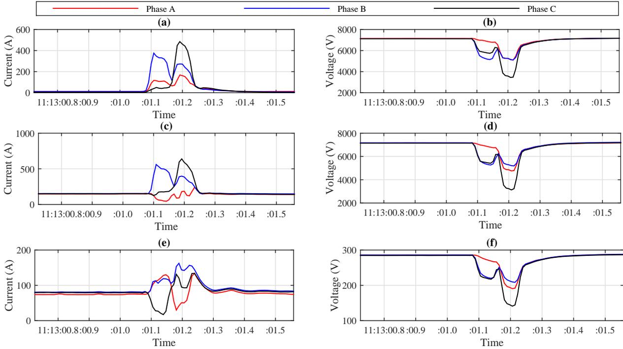
Fig. 4. Three phase voltage and current transients at the first lightning event: (a) and (b) Micro-PMU 1; (c) and (d) Micro-PMU 2; (e) and (f) Micro-PMU 3.
