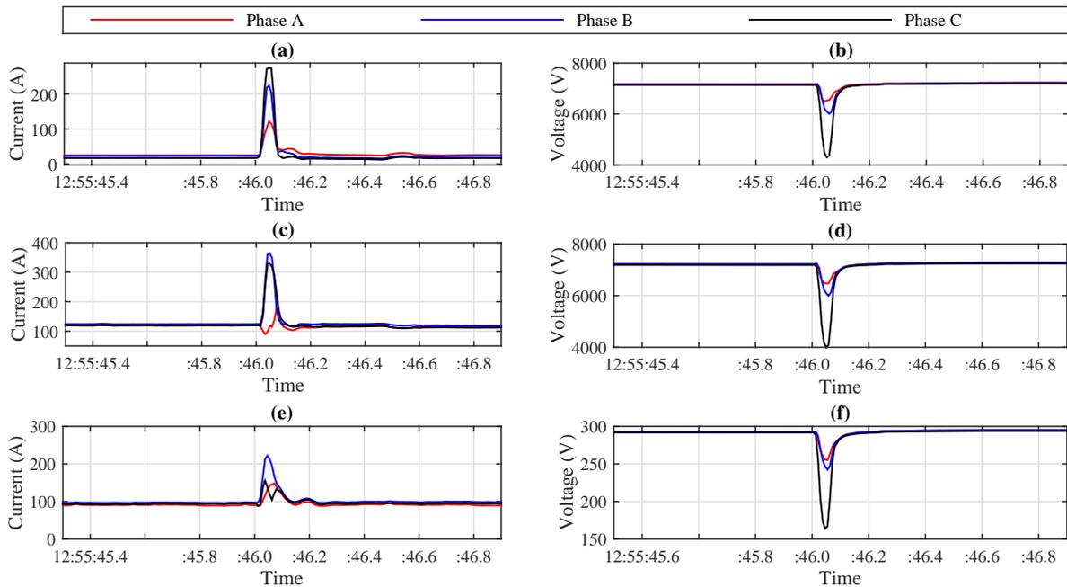
Fig. 8. Three phase voltage and current transients at the third lightning event: (a) and (b) Micro-PMU 1; (c) and (d) Micro-PMU 2; (e) and (f) Micro-PMU 3.
