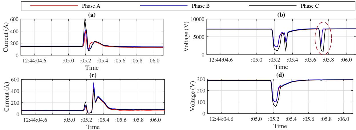
Fig. 7. Three phase voltage and current transients at the second lightning event: (a) and (b) Micro-PMU 2; (c) and (d) Micro-PMU 3.
