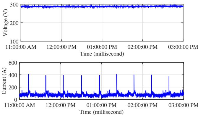
Fig. 3. Single phase voltage and current of Micro-PMU 3 for a four-hour period during a sunny day, October 25 2016, one day before the rainy day.
