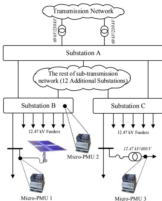
Fig. 1. The real-world test system that is studied in this paper is part of a sub-transmission system in Riverside, CA, which includes a PV farm under Substation B. Data from three Micro-PMUs are used for this analysis.
