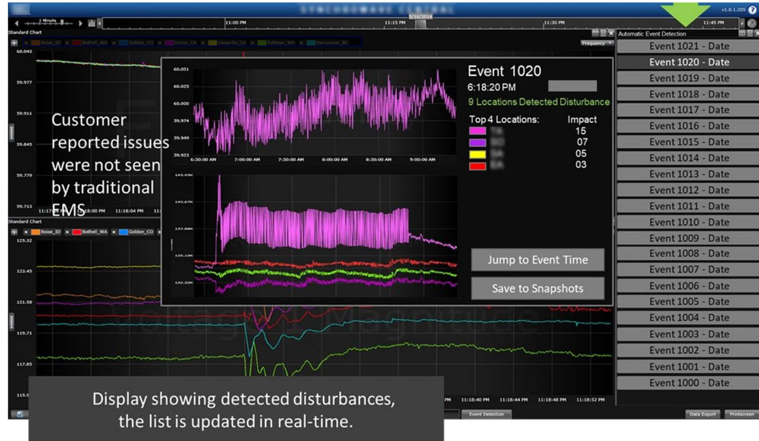
STATCOM Oscillation Captured by Engineering PMU Data Client System
