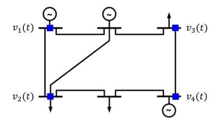
■ Waveform Measurement Unit (WMU)
