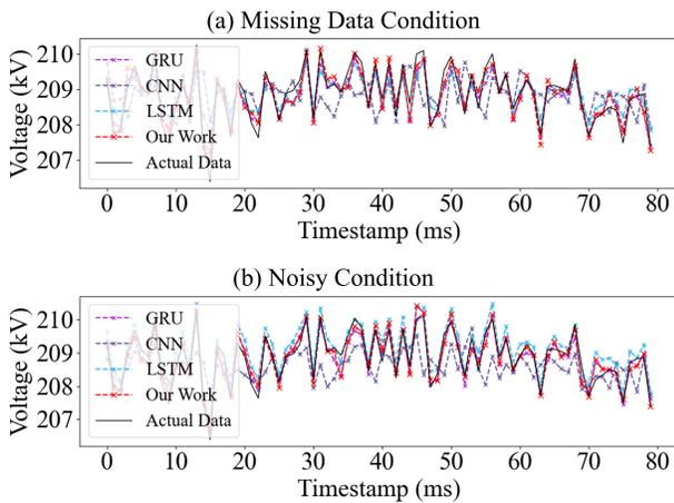
Fig. 5: Performance Comparison of Different Models under Missing Data and Noisy Conditions after Noisy Reduction.
