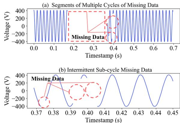
Fig. 1: Examples of Missing Data in Real-world Voltage Synchro-waveforms in a Pilot Testbed.
