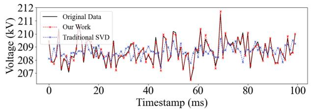
Fig. 4: Comparison of Waveform Completion Methods.
