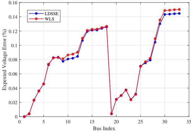
Fig. 6. The expected errors for the estimated nodal voltages phasor obtained from LDSSE and nonlinear WLS.
