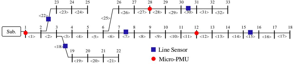
Fig. 1. The IEEE 33 bus test system that is used in our case studies. Three micro-PMUs are deployed on buses 1, 12, 28; and five line current sensors are deployed on line segments <7>, <15>, <18>, <22>, and <30>.
