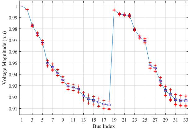
Fig. 2. Accuracy of voltages magnitude estimated by LDSSE in IEEE 33 bus test system.
