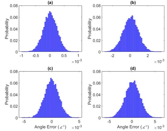
Fig. 5. Probability distribution of errors for estimated voltages angle at buses (a) 3, (b) 11, (c) 19, and (d) 33.
