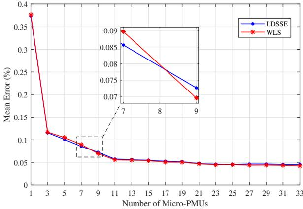
Fig. 8. Performance comparison of both LDSSE and WLS methods against number of deployed micro-PMUs in the test feeder.
