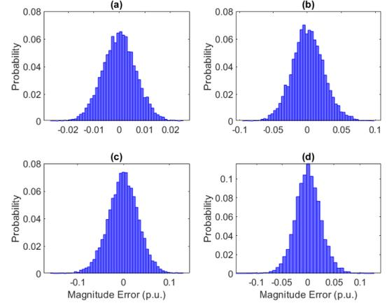
Fig. 4. Probability distribution of errors for estimated voltages magnitude at buses (a) 3, (b) 11, (c) 19, and (d) 33.
