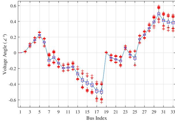
Fig. 3. Accuracy of voltages angle estimated by LDSSE in IEEE 33 bus test system.
