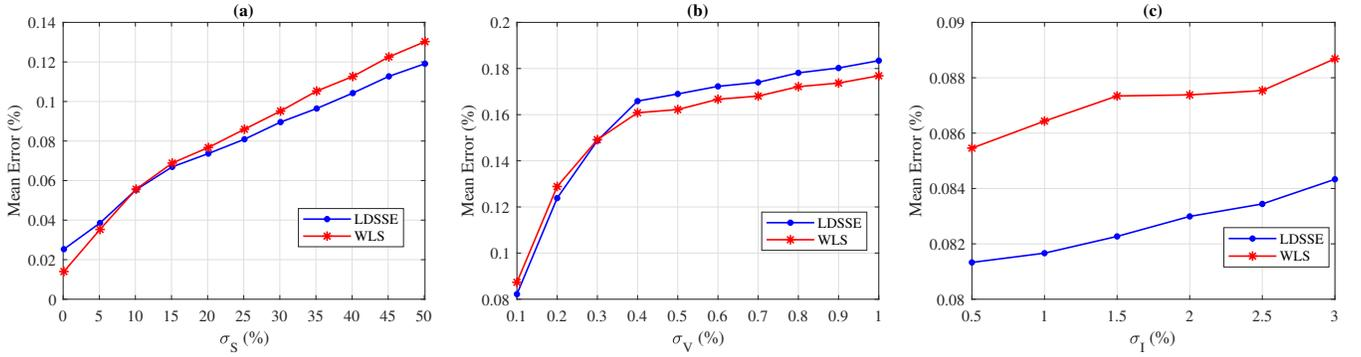
Fig. 7. Performance comparison of both LDSSE and WLS methods against: (a) pseudo-measurement accuracy; (b) micro-PMU measurement accuracy; (c) line current measurement accuracy.
