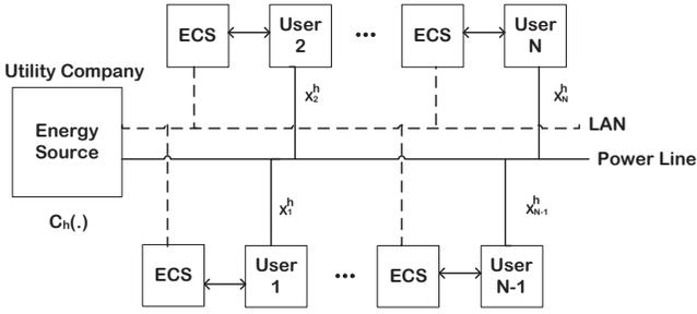
Fig. 1. A power system of  $N$  users and one shared energy source. Each user can be equipped with an ECS unit to participate in autonomous DR.
