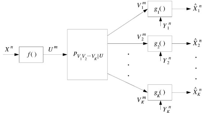
Fig. 1. Slepian–Wolf coding over broadcast channels. The achieved rate is  $\kappa = \frac{m}{n}$  channel uses per symbol.
