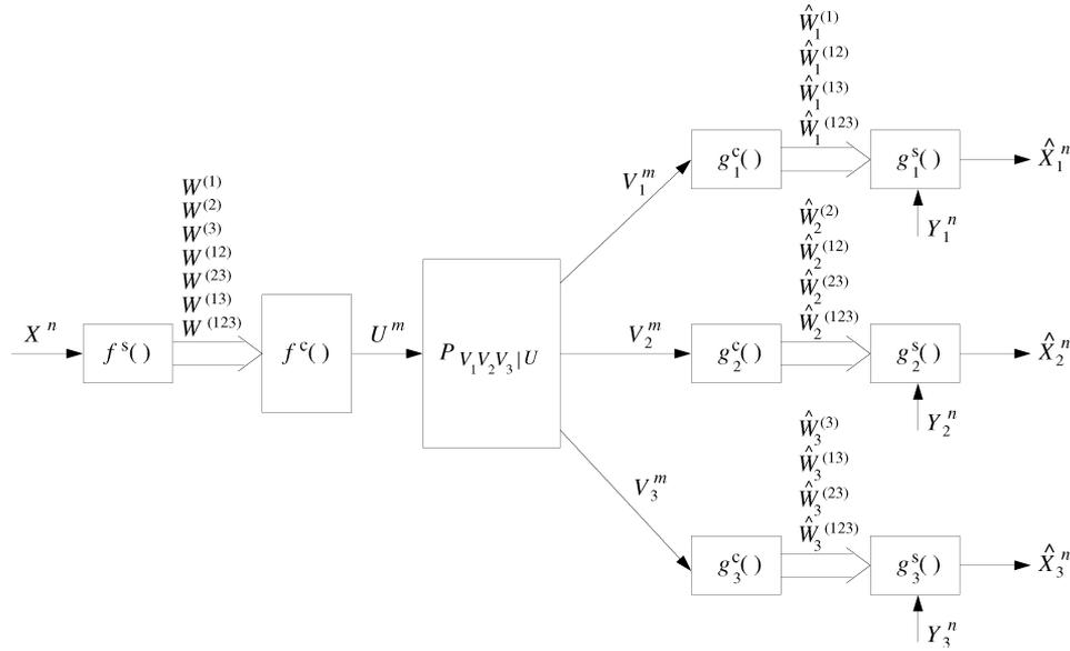
Fig. 2. Separation with stand-alone source and channel coders for  $K = 3$ . At the output of the source encoder  $f^s(\cdot)$ , there are seven distinct messages intended for different sets of decoders. For example, message  $W^{(13)}$  is for receivers 1 and 3 only, and  $\hat{W}_1^{(13)}$  and  $\hat{W}_3^{(13)}$  are its reconstructed versions at channel decoders  $g_1^c(\cdot)$  and  $g_3^c(\cdot)$ , respectively.
