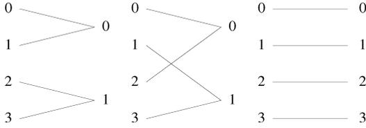
Fig. 5. A deterministic broadcast channel with  $\mathcal{U} = \{0, 1, 2, 3\}$ ,  $\mathcal{V}_1 = \mathcal{V}_2 = \{0, 1\}$ ,  $\mathcal{V}_3 = \{0, 1, 2, 3\}$ .
