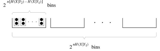
Fig. 3. Nested binning for  $K = 2$ . One can first create  $\approx 2^{nH(X|Y_2)}$  bins and group  $\approx 2^{n[H(X|Y_2) - H(X|Y_1)]}$  together to form a coarser binning with  $\approx 2^{nH(X|Y_1)}$  bins.
