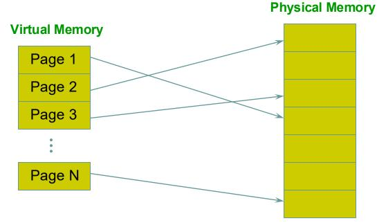
Paging solves the external fragmentation problem by dividing memory into fixed sized blocks that can placed anywhere in physical memory
