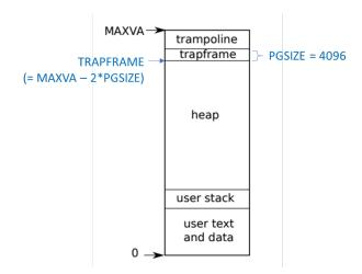
In the virtual address space, user text, data, and user stack are mapped at the bottom. At top, you can see two special pages are mapped: trampoline and trapframe, each has the size of PGSIZE (= 4096 bytes). The trampoline page maps the code to transition in and out of the kernel. The trapframe page maps the PCB's trapframe object so that it is accessible by a trap handler while in the user space (see Chapter 4 of the xv6 book for more details).
