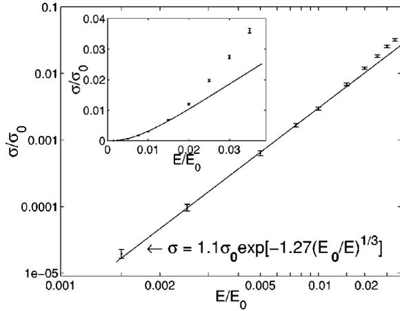
FIG. 1. The nonlinear dc conductivity  $\sigma = I/WE$  (normalized by  $\sigma_0 = I_0/WE_0$ ), as a function of electric field  $E$  for Model A. The straight line is the analytical fit discussed in the text. Inset: the same data on a linear scale.
