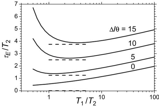
FIG. 1. The two-qubit entanglement duration  $\tau_E$  in units of the dephasing time  $T_2$  for the maximally entangled initial state ( $\beta = \pi/4$ ) and several values of the temperature  $\theta$ . Dashed lines correspond to Eq. (8).
