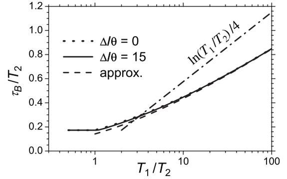
FIG. 2. The duration  $\tau_B$  of the Bell-CHSH-inequality violation (assuming  $\beta = \pi/4$ ) for  $\Delta/\theta = 15$  (solid line) and  $\Delta/\theta = 0$  (dotted line). The dashed line:  $\tau_B/T_2 = \ln[T_1/(4\tau_B)]/4$ .
