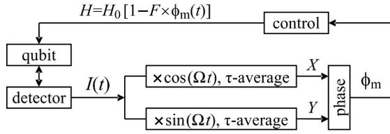
Fig. 1. Schematic of the proposed quantum feedback loop.
