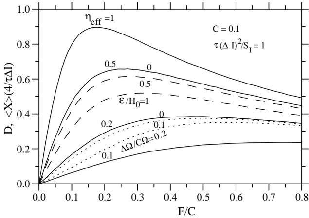
Fig. 3. Solid lines: synchronization degree  $D$  (and in-phase current quadrature  $\langle X \rangle$ ) as functions of  $F$  for several values of the detection efficiency  $\eta_{\text{eff}}$ . Dashed and dotted lines illustrate the effects of the energy mismatch ( $\epsilon \neq 0$ ) and the frequency mismatch ( $\Omega \neq \Omega_0$ ).
