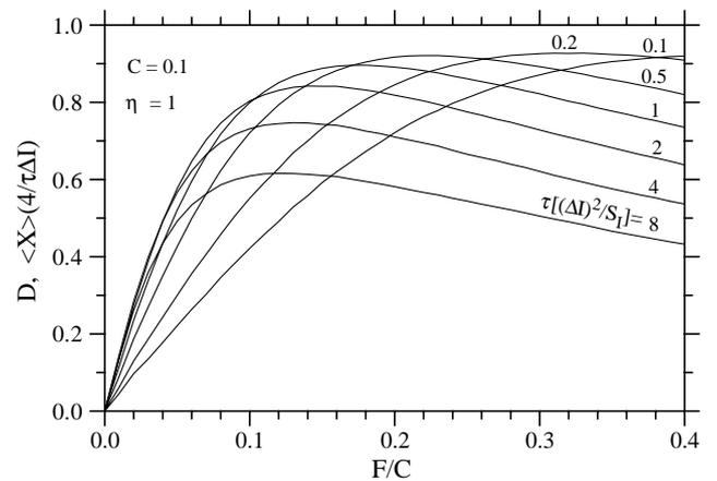
Fig. 2. Dependence of the synchronization degree  $D$  on the feedback factor  $F$  in ideal case ( $\gamma = 0$ ) for several  $\tau$ . Experimentally  $D$  can be measured via average in-phase current quadrature  $\langle X \rangle$ .
