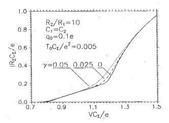
FIG. 4. Large scale I-V curves of the SET for three values of overheating parameter  $\gamma=0, 0.025$ , and 0.05. The heat drain is described by Eq. (16).
