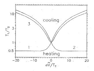
FIG. 2. Illustration of the possibility of cooling due to the tunneling. The curves separate regions of heating and cooling of the "first" electrode of the tunnel junction biased by the voltage  $\tilde{V}$ . Curve 1 corresponds to tunneling only from the first electrode to the second one, curve 2 corresponds to tunneling in the opposite direction, and curve 3 takes both processes into account.
