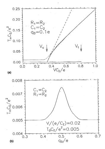
FIG. 3. Electron temperature  $T_m$  of the thermally isolated middle electrode of the SET as a function of (a) the voltage V, and (b) the background charge  $q_0$ . In (a) the solid line corresponds to  $T_0=0$ , the dotted line to  $T_0=0.01e^2/C_{\Sigma}$ , and the dashed line shows the analytical result [Eq. (22)].
