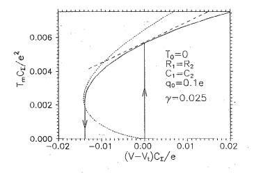
FIG. 5. The hysteretic  $T_m(V)$  dependence in the vicinity of the Coulomb blockade threshold  $V_t$  for  $\gamma=0.025$  and  $T_0=0$ . The dotted line corresponds to Eq. (25), the dashed line to Eq. (29).
