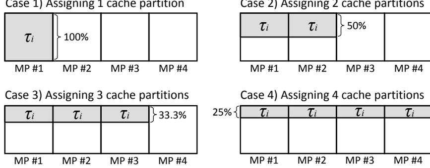
Figure 7: Page allocations for different cache allocation scenarios
