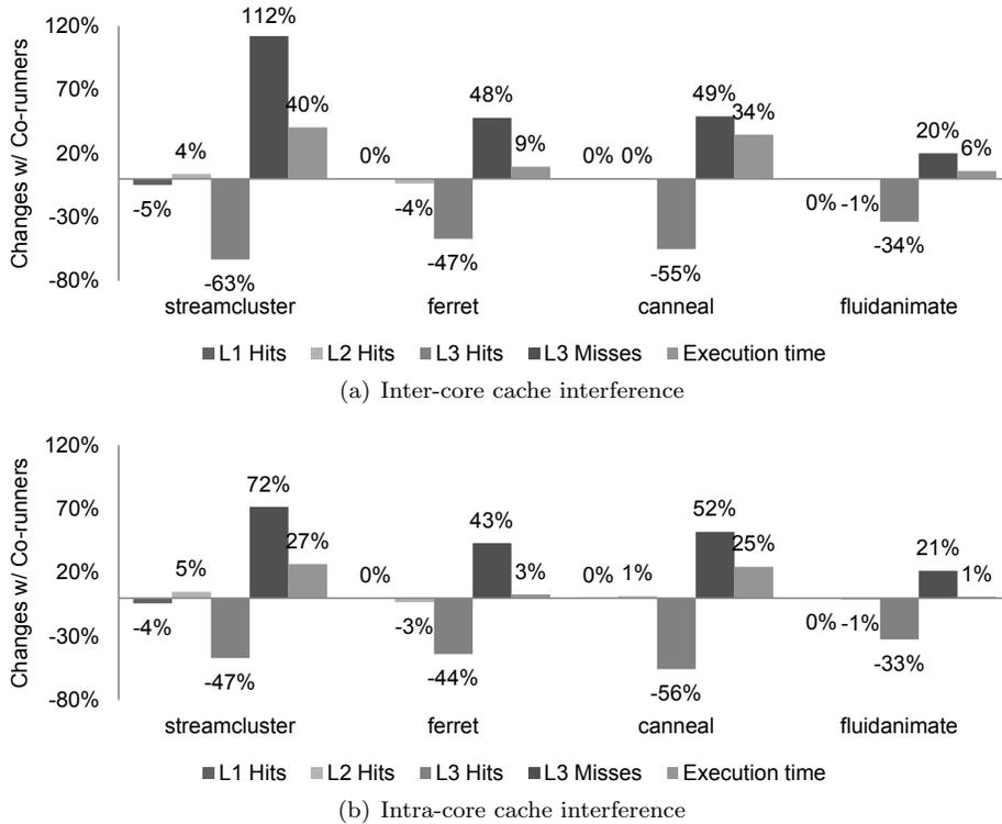
Figure 3: Performance changes due to cache interference
