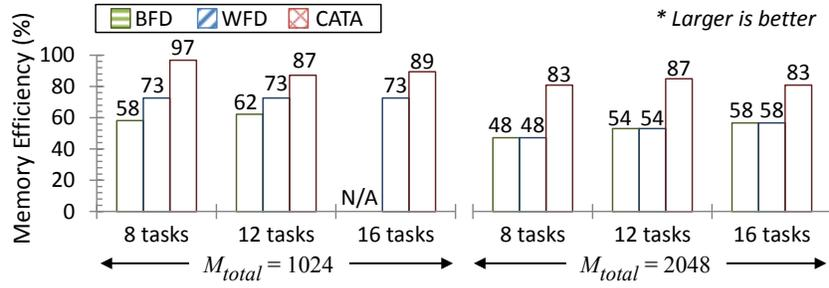
Figure 15: Memory space efficiency at minimum cache usage
