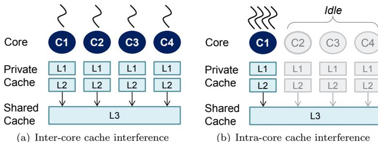
Figure 2: System configuration for cache interference measurement
