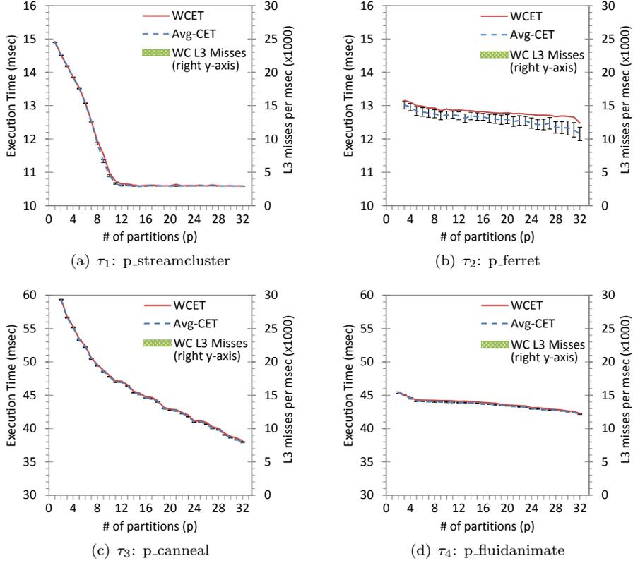
Figure 10: Execution time and L3 misses of each task as the number of cache partitions increases when running alone in the system
