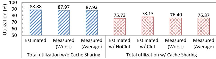
Figure 13: Total CPU utilization with and without cache sharing
