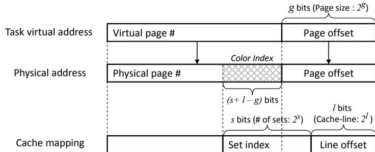
Figure 1: Memory to cache mapping and page coloring
