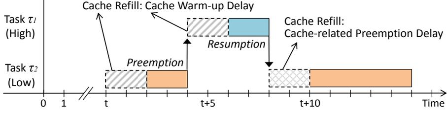
Figure 5: Cache warm-up delay and cache-related preemption delay
